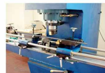
螺桿校直 Ball screw straighten
